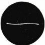
No. 3 — This oscillogram shows the small variation of resistance with varying voltage with an Allen-Bradley composition fixed resistor when an alternating E.M.F. is applied. Note how closely the Allen-Bradley resistor approximates the performance of a wire-wound resistor.
