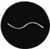
No. 2 — This oscillogram shows the wide changes of resistance with variations in voltage obtained in testing an average composition unit; note how inferior is its performance when compared with the Allen-Bradley fixed resistor as shown in oscillogram No. 3.
