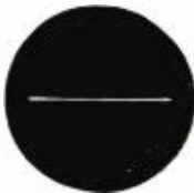
No. 1 — This oscillogram shows the constancy of resistance with varying potentials across the terminals of a wire-wound type of resistor, using an alternating E.M.F. Note how closely oscillogram No. 3 of an Allen-Bradley resistor approximates this performance.
